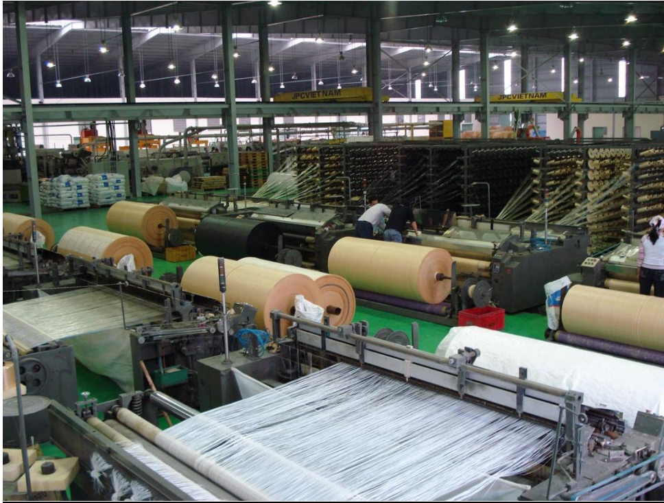
[ Water Jet Lines ]
